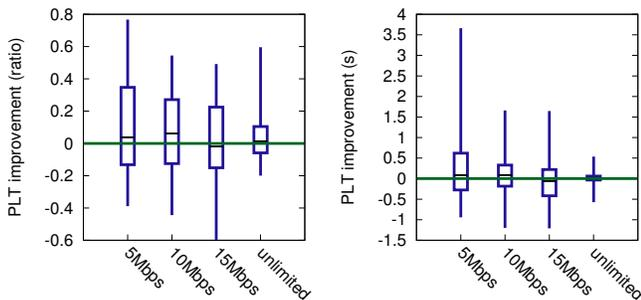
**Figure 9: Impact of bandwidth at 30ms latency.**
