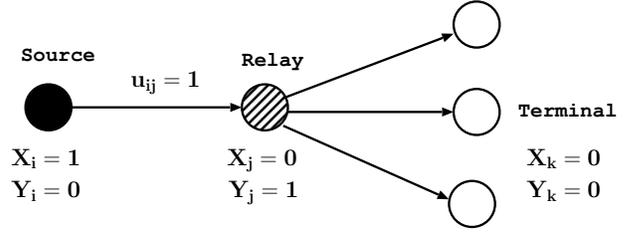
Fig. 2: Two-hop Relay Routing: node  $i$  is a source node ( $X_i = 1$ ), node  $j$  is a relay ( $Y_j = 1$ ), downloading traffic from  $i$  ( $u_{ij} = 1$ ), relaying video to other terminal nodes ( $X_k = Y_k = 0$ ).
