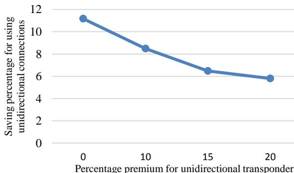
Fig. 5: Percentage saving of overall network cost as function of unidirectional port cost.
