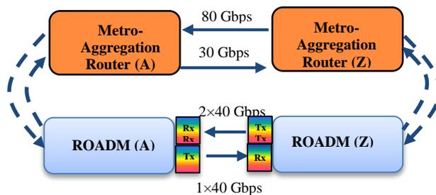
Fig. 3(b) Example of network planning for a metro-link between A and Z when unidirectional equipment is used.
