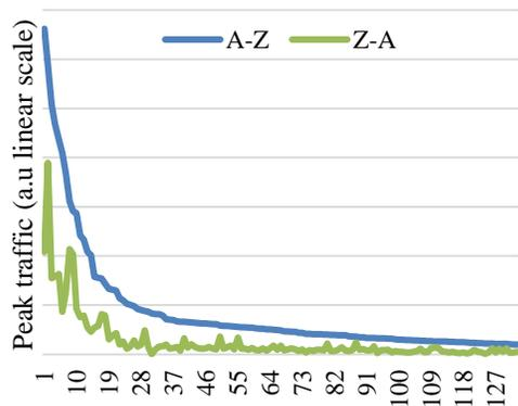
Fig.1 Peak traffic measured over one week interval on links of a particular metro area network. The network symmetric ratio for this metro area network was calculated as  $\rho_{network}=0.5$
