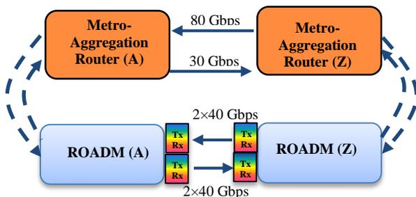
Fig. 3(a) Example of network planning for a metro-link between A and Z when bidirectional equipment is used.
