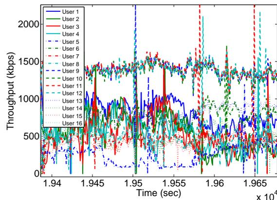
Fig. 9. Throughput v. time for Scenario 2c, 3 sectors, 16 UEs
