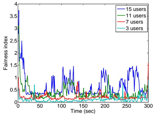
Fig. 5. Fairness index v. time for Scenario 1a (air-interface bottleneck)
