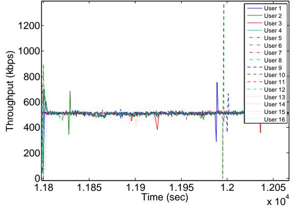
Fig. 7. Throughput v. time for Scenario 1c, 3 sectors, 16 UEs
