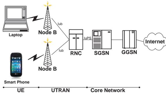
Fig. 1. UMTS network architecture
