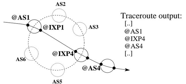
Figure 1: A typical IXP architecture with 6 AS members.
