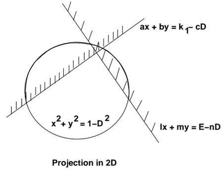
Figure 3: Reduction of overlap test to the plane
