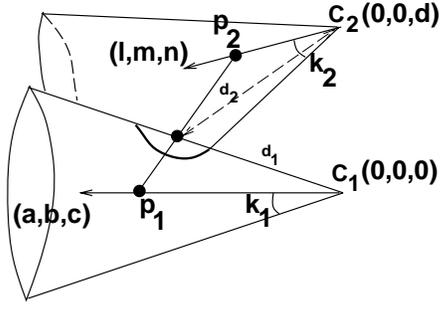
Figure 5: Cone/Cone intersection
