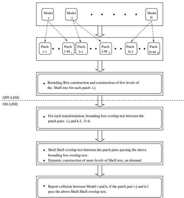
Figure 7: Overall Algorithm for Contact Determination
