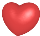
Figure 12: General Implicit Model: The image shows a heart-shaped implicit model polygonized using extended dual contouring. This model is represented as a sixth order implicit polynomial function.
